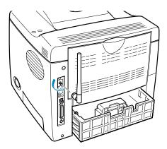
9 Connect the network or serial cable, reconnect the power cord and then turn the printer on.
